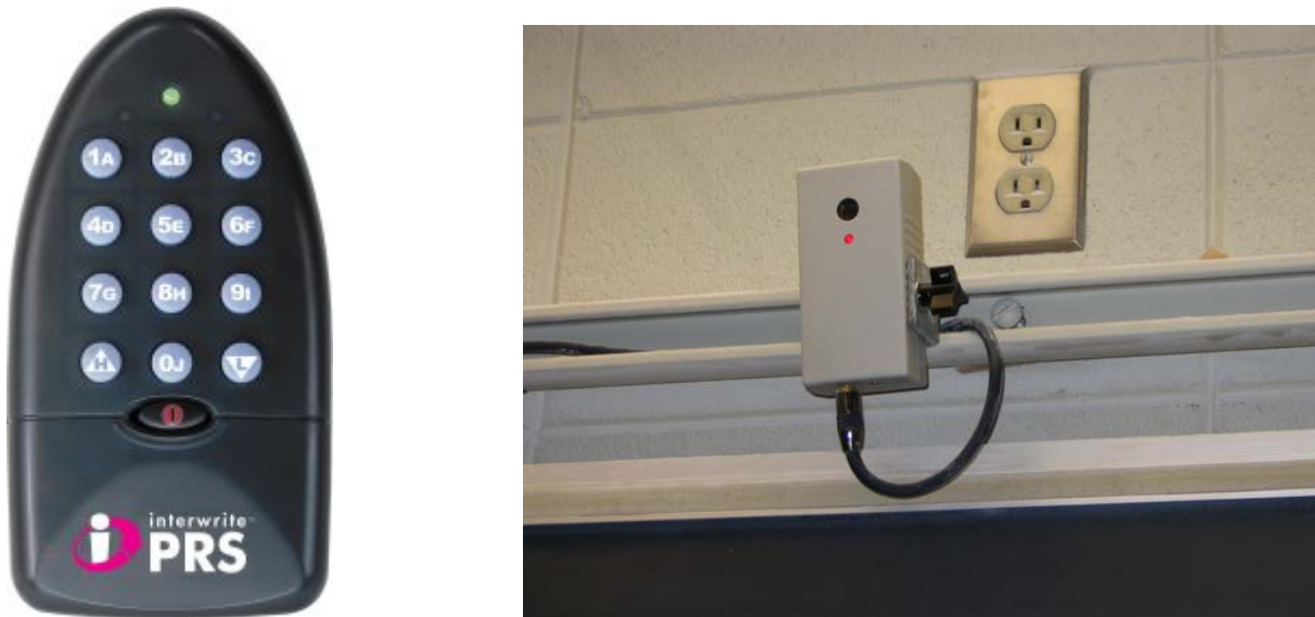
Fig. 1: The handheld RF transmitter (left) and one of two RF receivers installed in GSC 201. The receiver is linked to the smart classroom PC.
